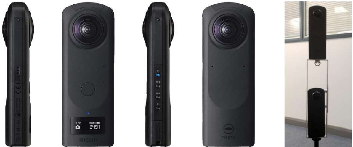
Figure 2.11: Ricoh Theta 360° and the stereo setup used in our experiments. ©Ricoh Company, Ltd. (the first 4 images). The last image was acquired by our collaborator Hansung Kim in the University of Surrey.
