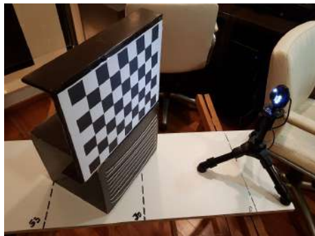
Figure 2.6: Calibration object used in the experiments.
