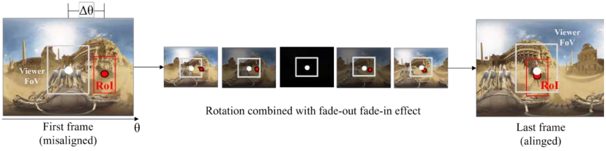
Figure 4.1: Fade-rotation alignment edit aligns the RoI with viewer FoV. For simplicity, we illustrate a fixed viewer FoV.
